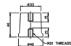
DETAILS OF SUPPORT INSULATOR FOR NEUTRAL BUS BAR (2 Nos.)
